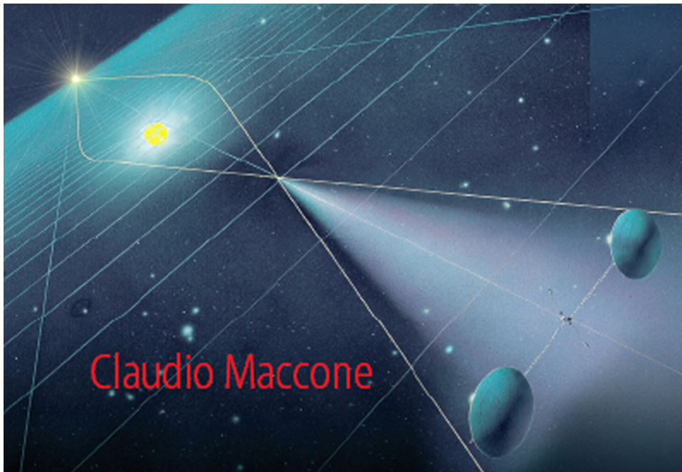
Figure 14.4: Enlarged part of the front cover of the author's 2009 book [19] showing: (1) the bright radio source at infinity (i.e. the horizon); (2) its radio waves flying by the Sun and made to focus at 550 AU; (3) the FOCAL spacecraft made up by two (say) 12-m antennae tied to each other by a tether and revolving in the orthogonal plane to the spacecraft's velocity vector. The same is shown here, with the two Archimedean Spirals covered by the antennae.
