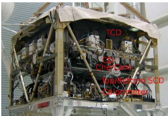
Figure 1: CREAM-III Instrument; From the top: TCD, CD, CherCam, top and bottom SCD, and Calorimeter.
