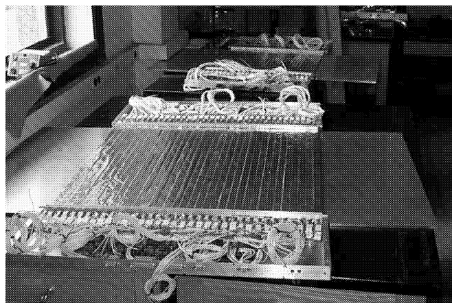
Figure 4: Bottom half of the S2 Hodoscope
